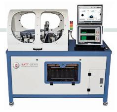
ASDI is a stationary fully automated diamond verification instrument, designed to screen large quantities of colourless and near colourless loose stones at a high speed. ASDI automatically separates diamonds from synthetic diamonds and diamonds simulants.
