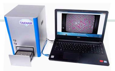
DiamondDect 5 is a desktop diamond verification instrument for mounted and loose stones, designed to separate diamonds from HPHT synthetic diamonds. DiamondDect 5 is manually operated but gives an automatic test result.
