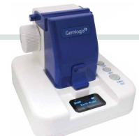
LEO is a portable desktop diamond verification instrument for loose and mounted stones, designed to separate diamonds from synthetic diamonds and diamond simulants. Leo is manually operated but gives an automatic test result.
