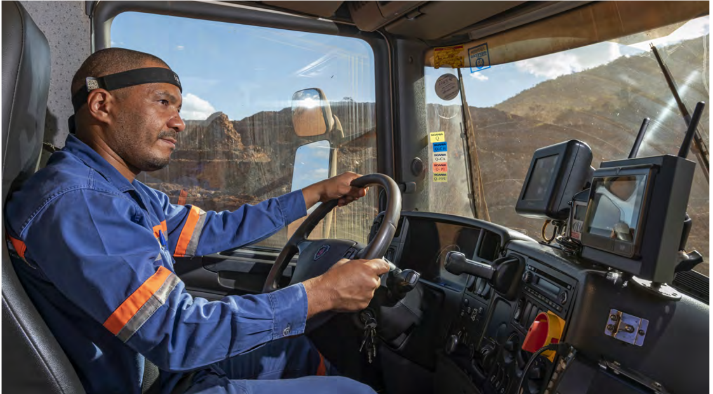
Our technical teams are leveraging technology to enhance safety through the deployment of advanced driver assistance systems (ADAS). Here, at our Barro Alto nickel operation in Brazil, mechanical engineer Odilson Ribeiro wears a fatigue-monitoring 'smart cap' specifically designed for haul-truck drivers.
